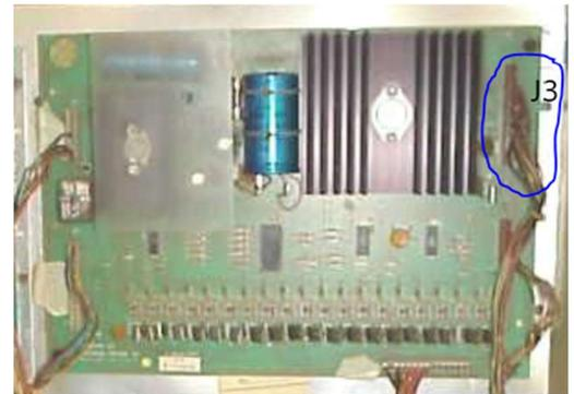
With your multi-meter, set to DCV measurement. Place the black test lead on the GND test-point and using the red test lead check each one of the other test-points. Voltages measured should be +/- 2V, with the exception of the +230V which should be ~+165V. It will measure ~+230V when you plug J3 into the Solenoid Driver Board.
